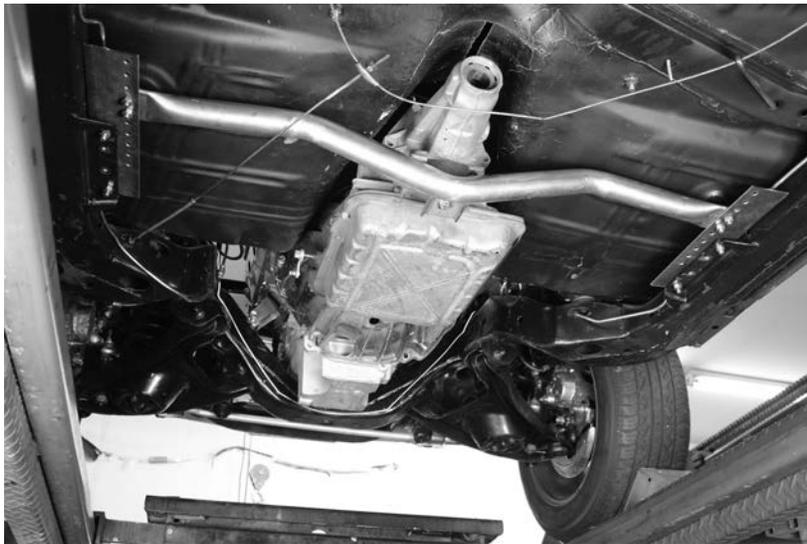
Install the crossmember frame brackets in the original bolt holes then mount the crossmember.
