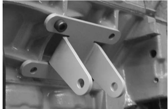
Start the 3/8"-16 nylon lock nuts and flat washers on the two studs that are attached to the frame brackets and through the frame but leave them loose at this time. After the assembly is in place slide the mounts into position.
