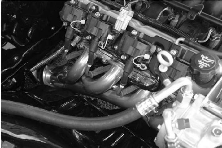
Mid length and long tube headers can now be installed with the engine in place.
