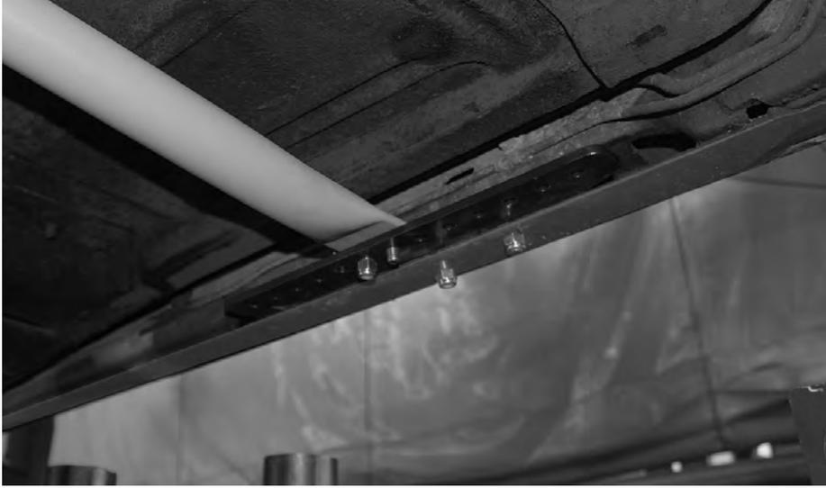
Mount the frame brackets to the frame through the original crossmember mounting holes. Then put the crossmember on top of the bracket.
