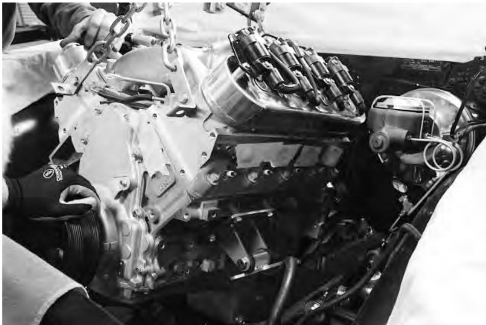
(Set the engine in place with each sides motor mount and frame bracket loosely on engine)
