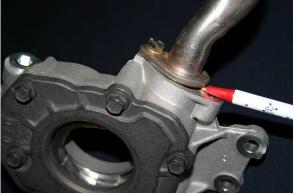
(This pickup tube is **NOT** installed correct)
