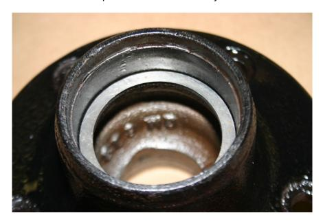
Now you can press in the large inner race on top of the bearing shim.
