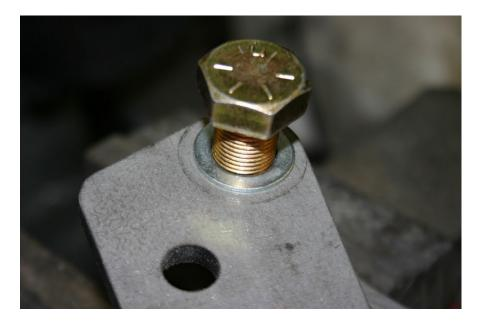
Tighten the 5/8" and ½" Bracket bolts. It is a good idea to use red loctite on the 5/8" bolt.
