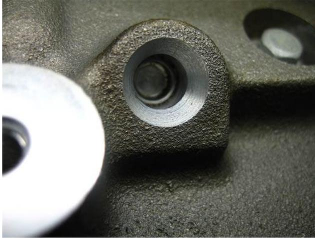
**Step 2:** Remove oil pump pickup tube and Windage tray, make sure the original oil pump pickup tube o-ring is removed. Install the new Windage tray and fasteners placing a drop of blue Loctite on the threads. Torque the fasteners to 106 in/lbs. Install the new pickup tube (and girdle if you ordered on with your oil pan), make sure that the pickup tube is installed correctly into the oil pump housing. Place a drop of blue Loctite on the threads and torque the fasteners to 106 in/lbs.
