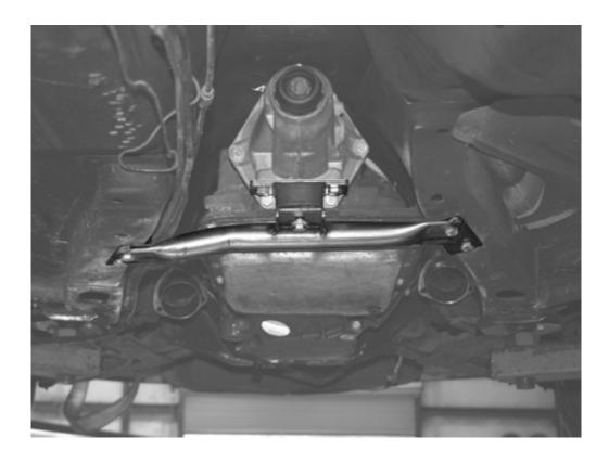
Using a jack to lift the transmission into position you can install the transmission crossmember using the 10mm bolts provided. Using the  $7/16"-13 \times 1"$  bolt and flat washer bolt the transmission mount to the crossmember.
