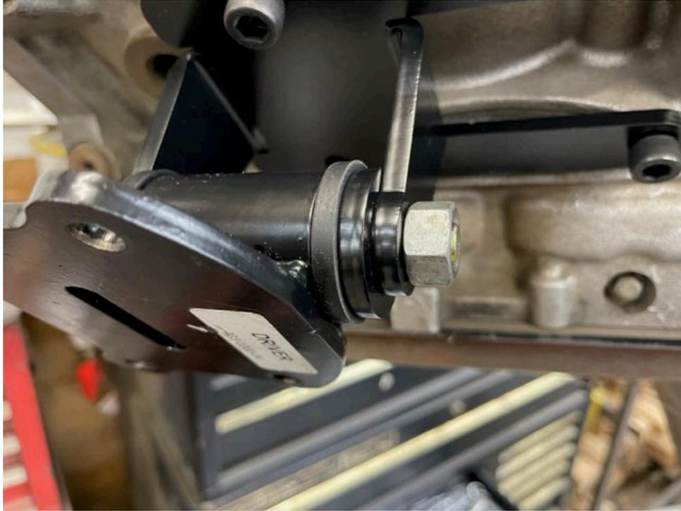
Notice the included  $\frac{1}{4}$ " thick washer that goes between the frame mount bushing and engine mount tab. This keeps the Bushing from wanting to push out of the frame mount under high loads.
