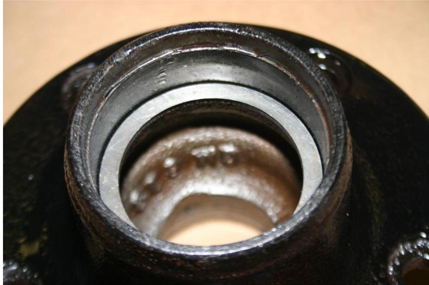
Now you can press in the large inner race on top of the bearing shim.
