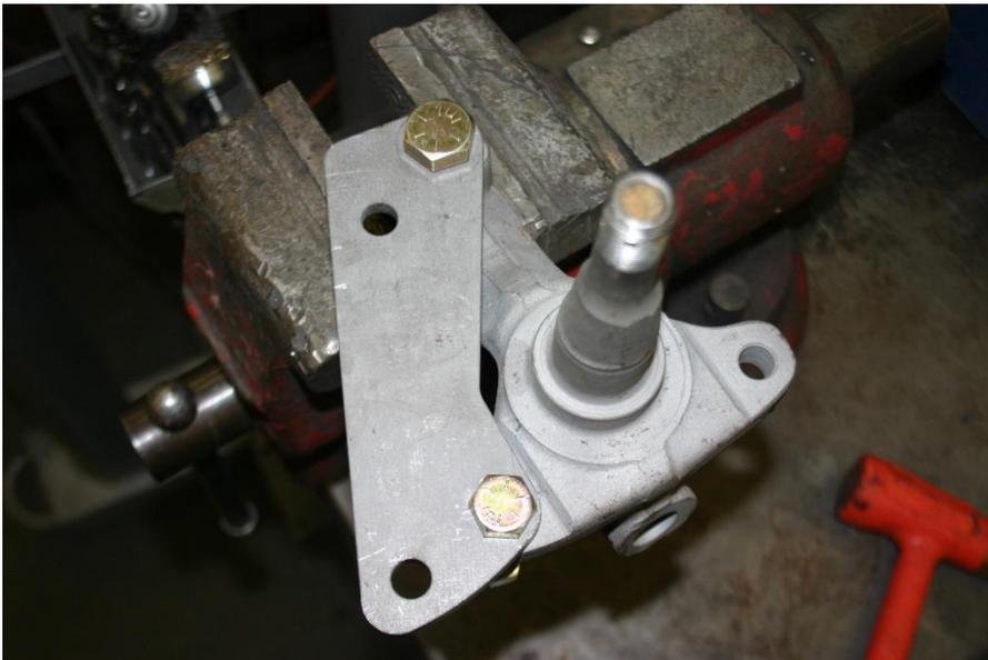
You will need to use the supplied 1/2" x 3" bolt in the rear steering arm bolt hole as the extra thickness of the bracket will make the factory one too short.
