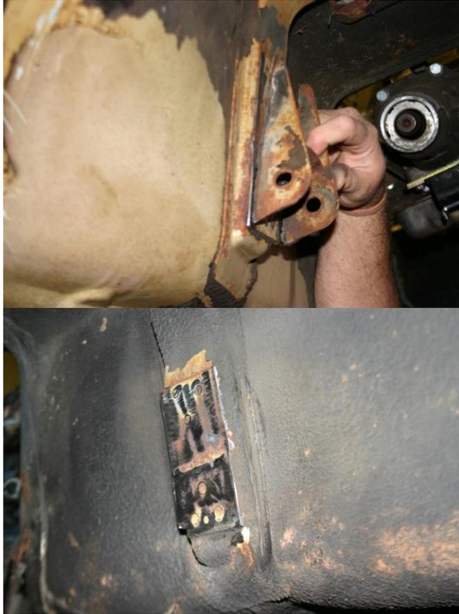
**Step2:** Position the transmission crossmember in the tunnel where the original crossmember tabs were removed, lining up the crossmember with the back edge of the original crossmember tabs. Mark the holes through the crossmember on the underside of the tunnel.
