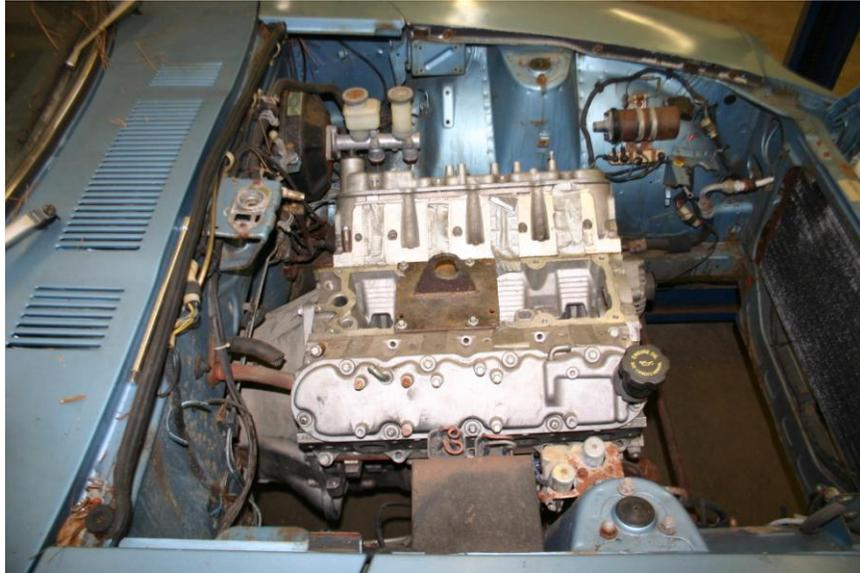
**Step 6:** Align the frame bracket to frame bolt holes and install the ½"-13 x 1" bolts and nylon lock nuts. After everything is lined-up tighten the motor mount to block bolts, the frame bracket to frame bolts and the engine mount to frame bracket bolts.
