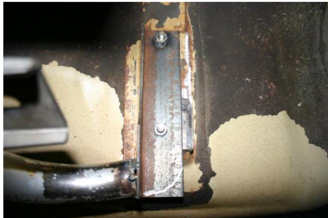
**Step 3:** Drill the holes with a 1/4" drill bit all the way through both layers of the tunnel floor **(make sure the carpet is removed prior to drilling)**. Using the 1/4" holes as a guide drill through the TOP layer of the floor from inside the vehicle using a 1" holesaw **(DO NOT DRILL ALL THE WAY THROUGH BOTH LAYERS OF THE FLOOR)**. Using a 25/64" drill bit drill through the remaining 1/4" hole.
