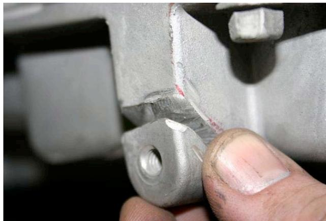
**Step 3:** Locate the motor mounts and loosely bolt them to the engine using the supplied 10mm allen head bolts. Now loosely bolt the Driver's Side (LEFT) and Passenger's Side (RIGHT) frame brackets to the engine mounts using the supplied 1/2"-13 x 4" long bolts and nylon lock nuts. (The bolts will be tightened after the engine is set in place and everything is lined-up)
