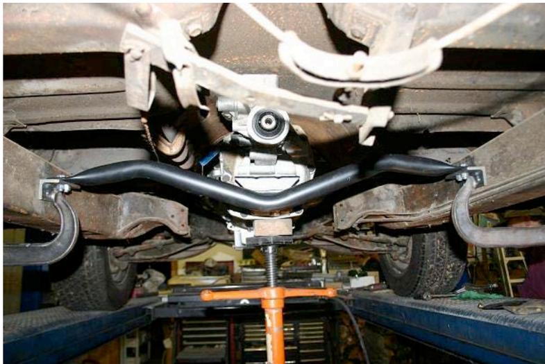
**Step 7:** Once you have snugged-up all of the bolts, check the clearance between the drag-link and the front of the oil pan. With the steering centered you should have approximately 2" of clearance, with the steering turned all the way to the left you should have approximately 3/8" of clearance.
