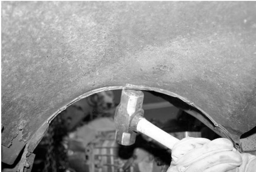
**Step 2:** The GM LH8 oil pan will require slight trimming to clear the 1955-1957 frames. The part that needs to be trimmed is highlighted in the first photograph. The second photo details how much needs to be trimmed.
