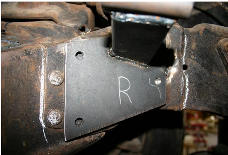
(Detailed view of driver's side frame bracket on the frame)
