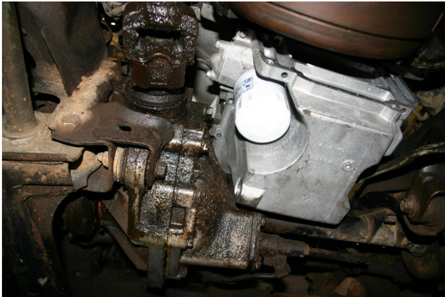
(This pictures shows the clearance between the oil pan and the front differential)
