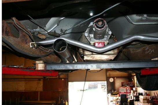
**Step 5:** Once you have checked to make sure that everything is installed correctly and lined up go back and tighten the engine mount to block bolts, engine mount to frame bracket bolts, frame bracket to frame bolts, transmission mount to transmission bolts, transmission mount to crossmember bolts and transmission crossmember to frame bolts.
