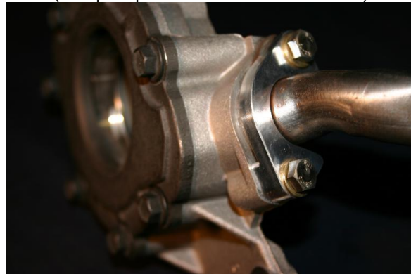
(This pickup tube is installed using our pickup tube girdle which uses
