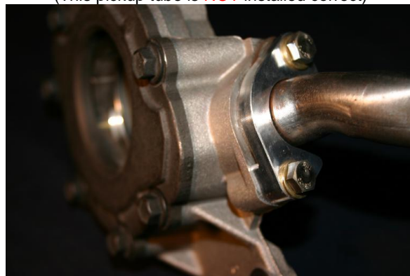
(This pickup tube is installed using our pickup tube girdle which uses two bolts to make sure the tube is squarely installed in the oil pump)
