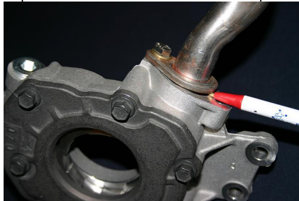
(This pickup tube is NOT installed correct)
