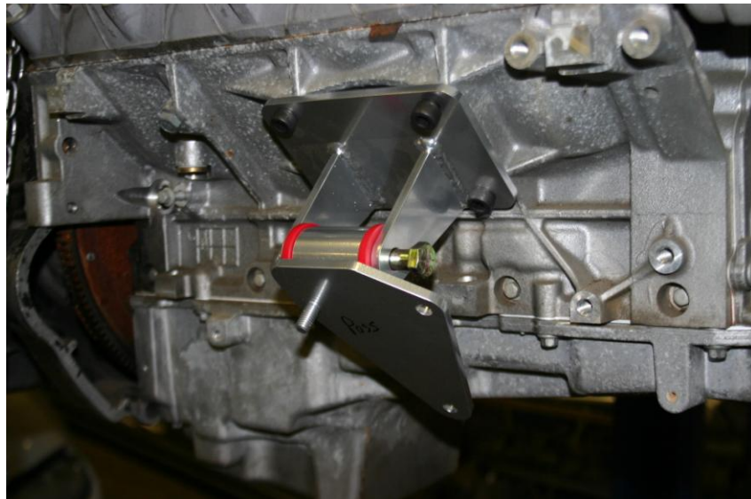
(Detailed view of passenger's side motor mount and frame bracket on engine)
