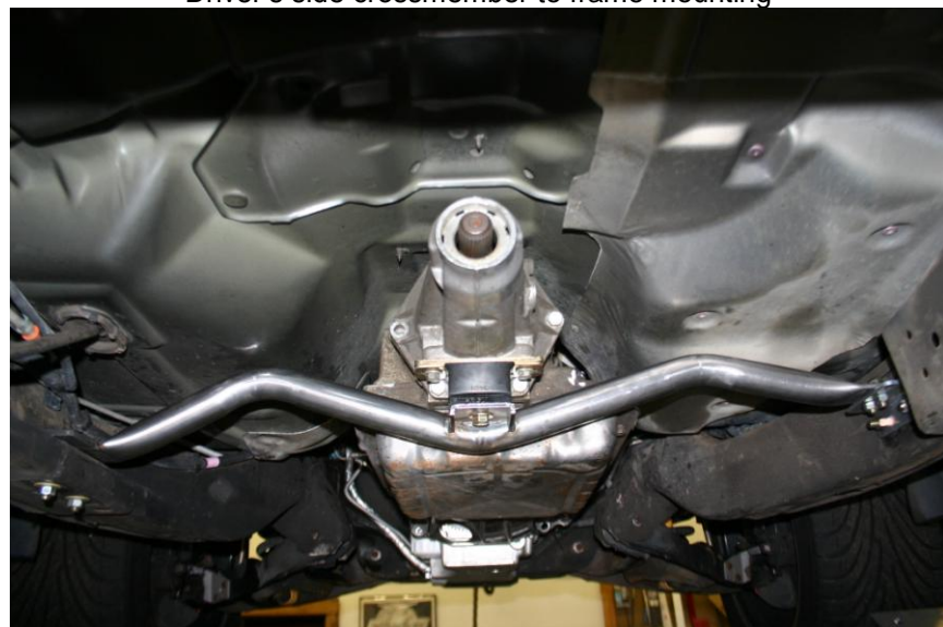
Transmission, crossmember & mount installed
