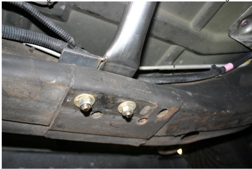
Driver's side crossmember to frame mounting
