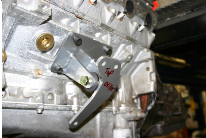
(Detailed view of driver's side motor mount and frame bracket on engine)
