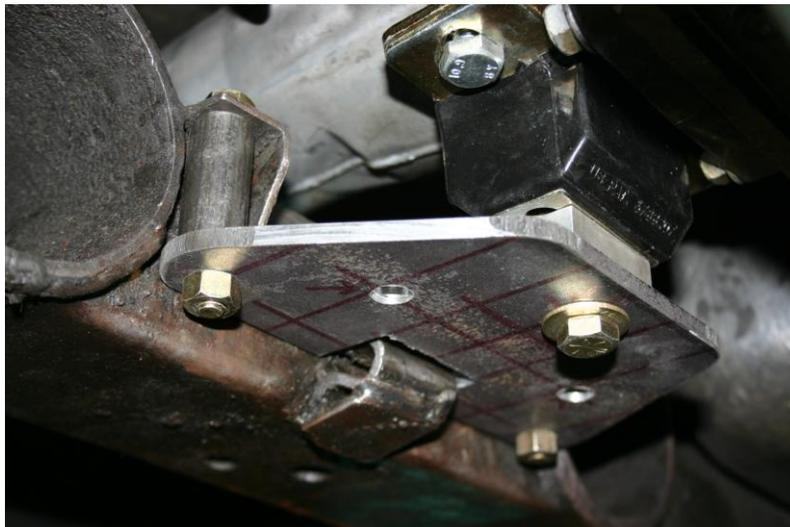
View of transmission bracket installed on Crossmember (this shows a 4L60E transmission, the T-56 transmission uses the back two bolt holes for mounting)
