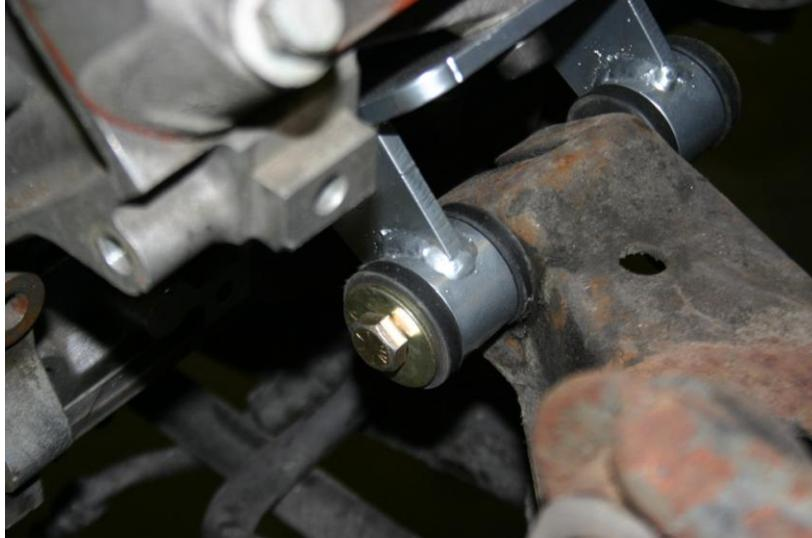
**Step 3:** Lift the rear of the transmission using a floor jack. Install the polyurethane transmission mount on the transmission, making sure that you install the provided plate between the mount and the transmission (this preloads the polyurethane mount).
