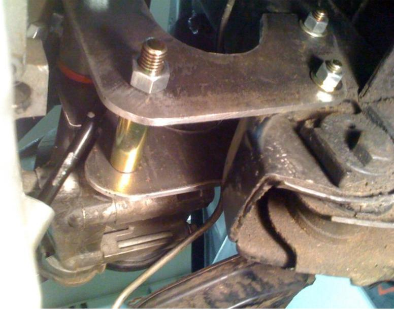
Here you can see how the dipstick tube runs through the notch in the mounting bracket. You may need to bend the dipstick tube slightly to get it to fit correctly.
