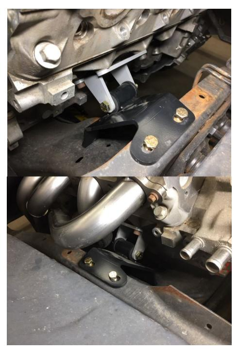
With the engine and frame mounts loosely bolted into the chassis, you can now install the Crossmember to the frame rails of the chassis. The transmission you have chosen will determine the fore and aft location of the Crossmember outer support brackets. The height of the brackets should be 2.5" from the bottom of the bracket to the bottom of the frame lip as shown in the photo. Use a 3/8" drill bit to drill the new holes to bolt the brackets to the chassis.
