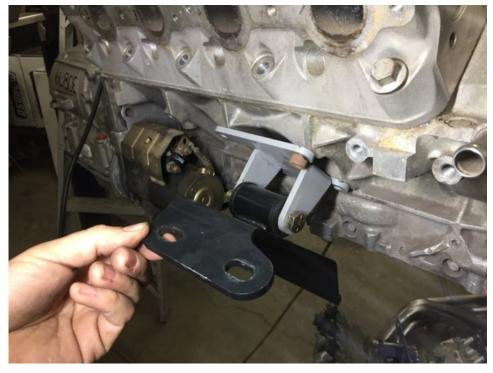
Lower the engine into the chassis aligning the engine mounts over the frame mounts and loosely install the  $\frac{1}{2}$ "-13 x 3.75" bolts, and nylon lock nuts. (you will have to support the rear the transmission in order to get the long  $\frac{1}{2}$ " bolts to slide in all the way through the engine and frame mount assembly)
