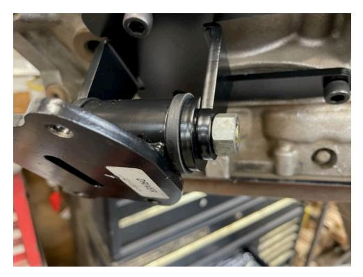
Notice the included ¼" thick washer that goes between the frame mount bushing and engine mount tab. This keeps the Bushing from wanting to push out of the frame mount under high loads.
