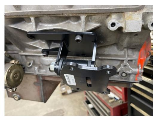
Detailed view of passenger's side motor mount and frame bracket on engine
