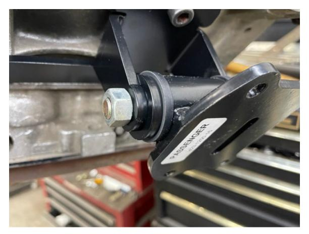
Notice the included ¼" thick washer that goes between the frame mount bushing and engine mount tab. This keeps the Bushing from wanting to push out of the frame mount under high loads.
