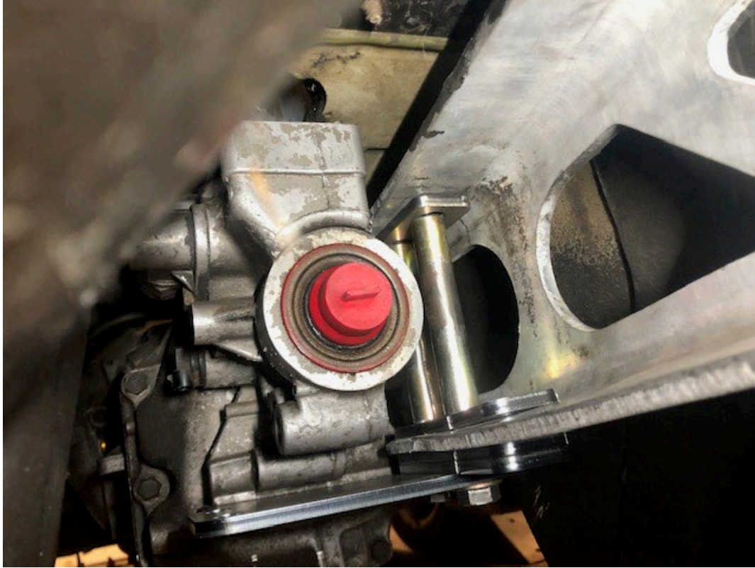
This photo shows a T56 transmission, note the positions of the three 1/4" shims. Two on the bottom of the c beam and one on top.
