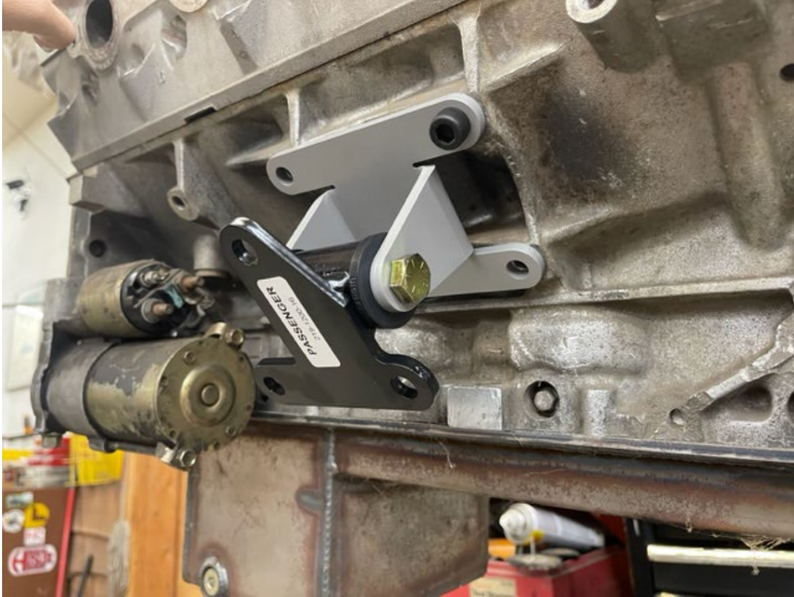
(Detailed view of passenger's side motor mount and frame bracket on engine)
