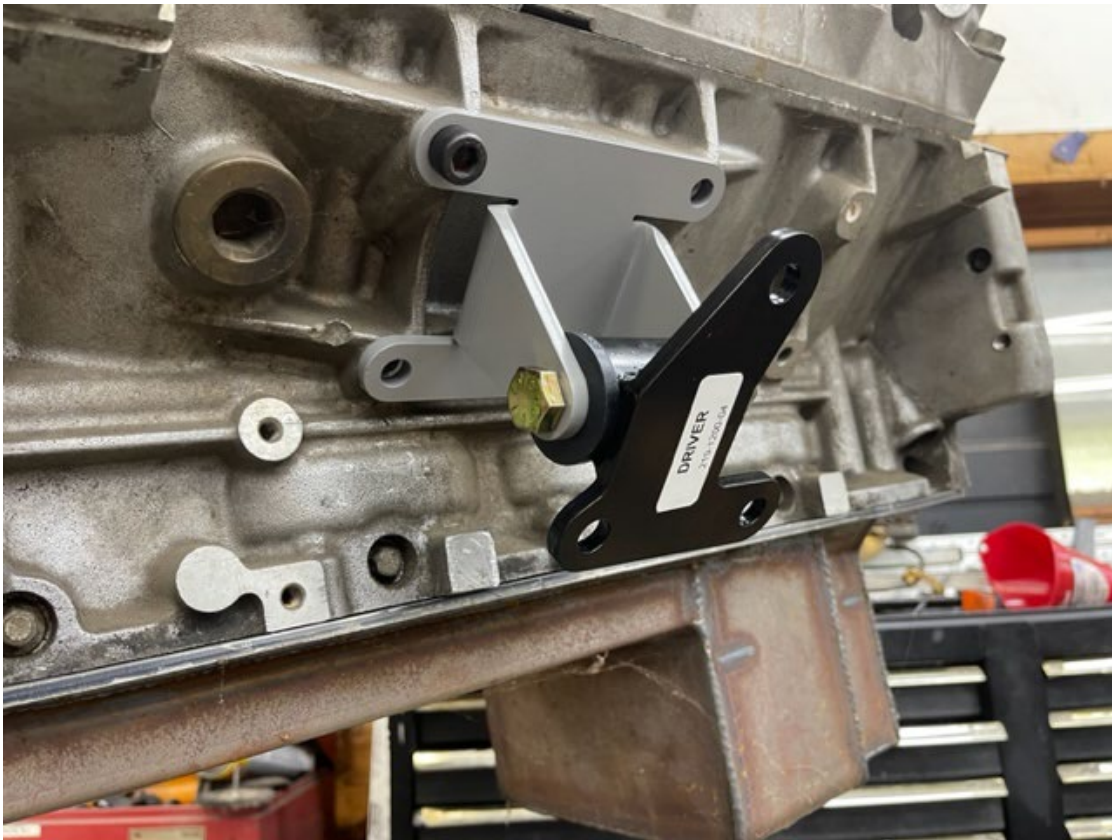
(Detailed view of driver's side motor mount and frame bracket on engine)
