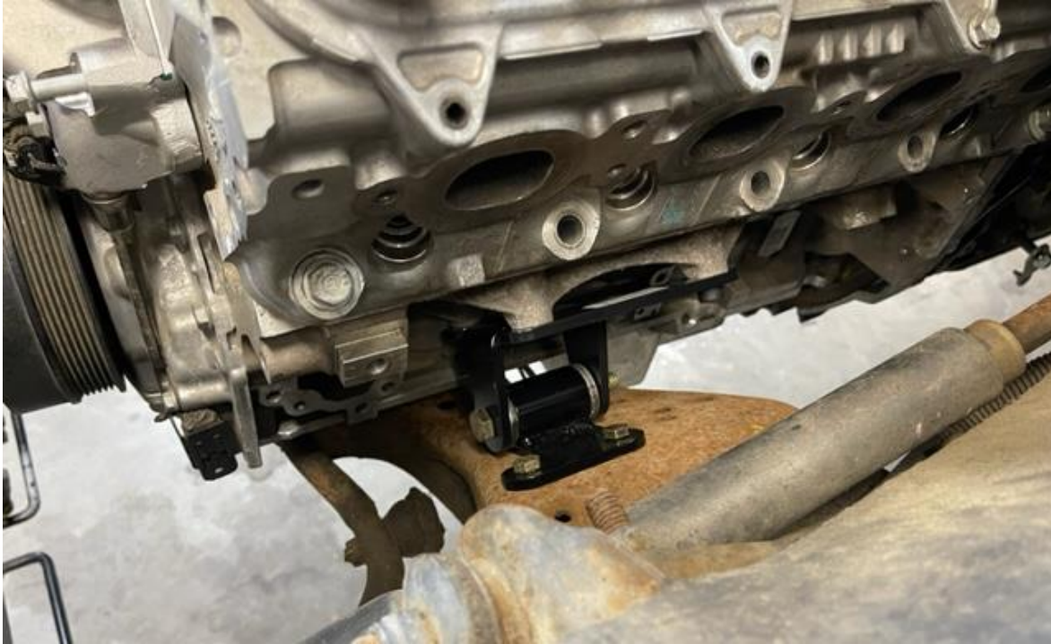
View of Driver side engine and frame mount
