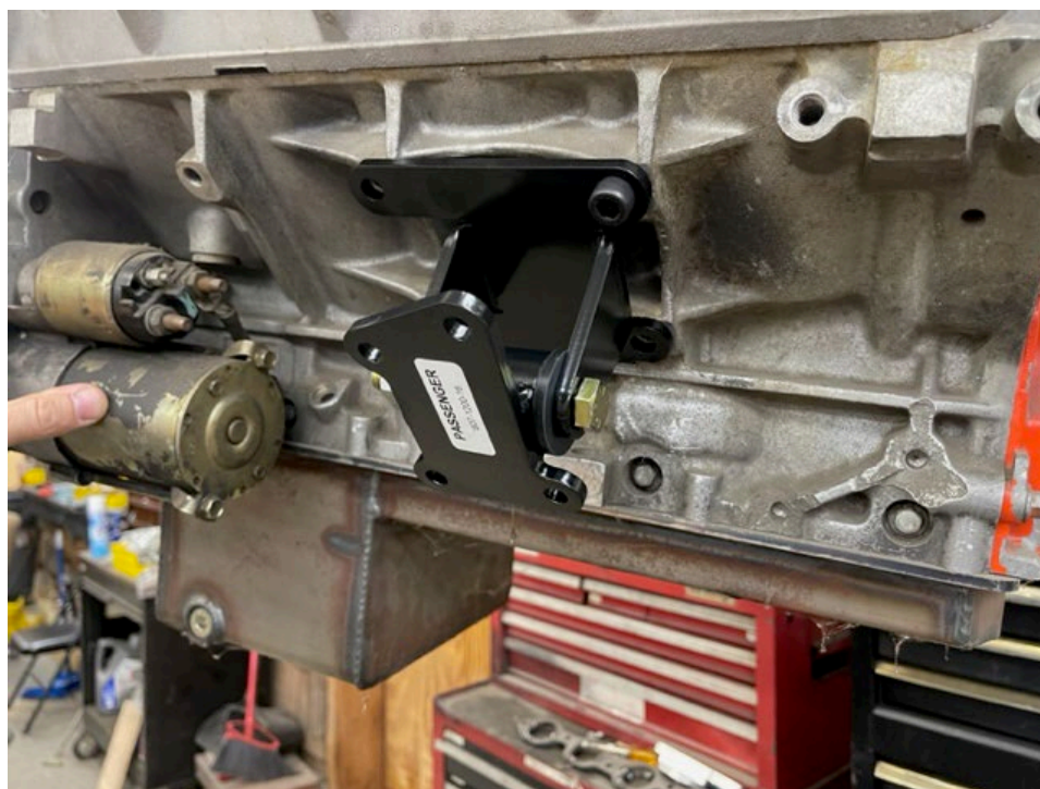
Detailed view of Passenger side engine mount and frame bracket on engine
