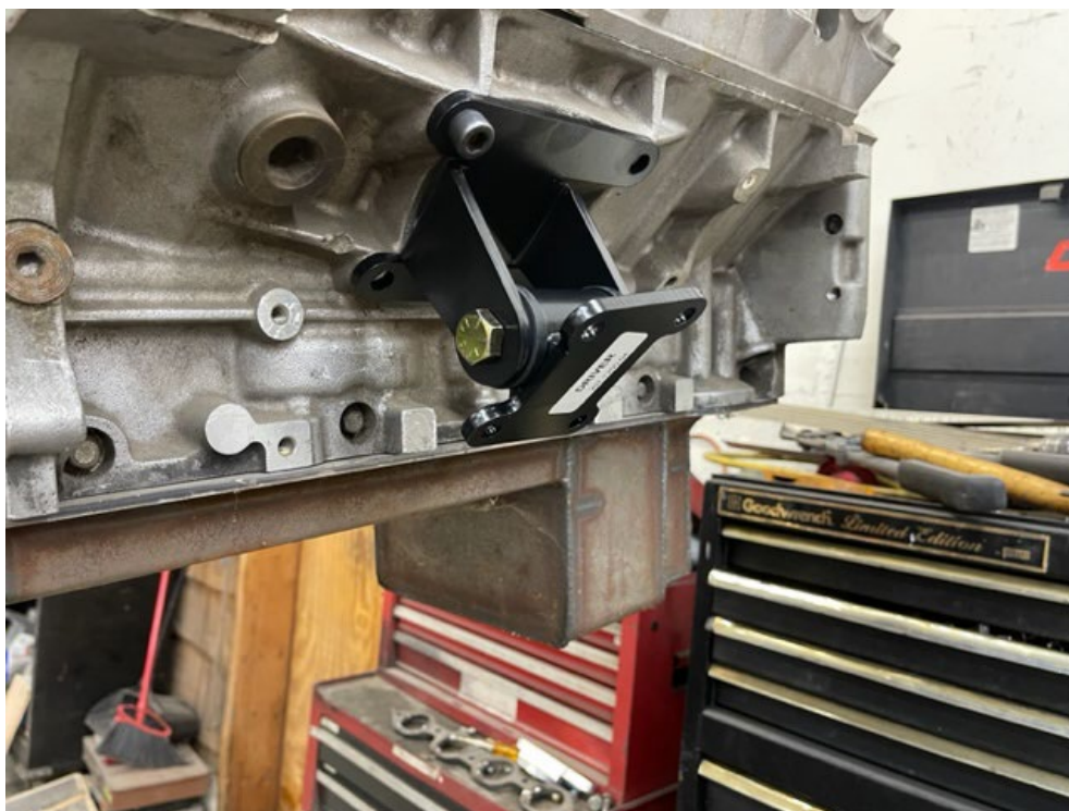
Detailed view of driver's side engine mount and frame bracket on engine
