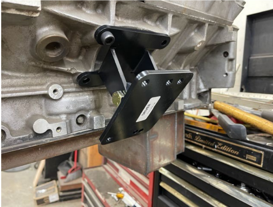
View of Driver side engine and frame mount (note orientation of both engine and frame mount)
