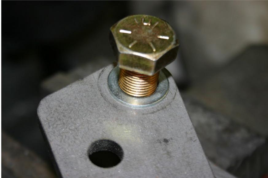
Tighten the 5/8" and 1/2" Bracket bolts. It is a good idea to use red loctite on the 5/8" bolt.
