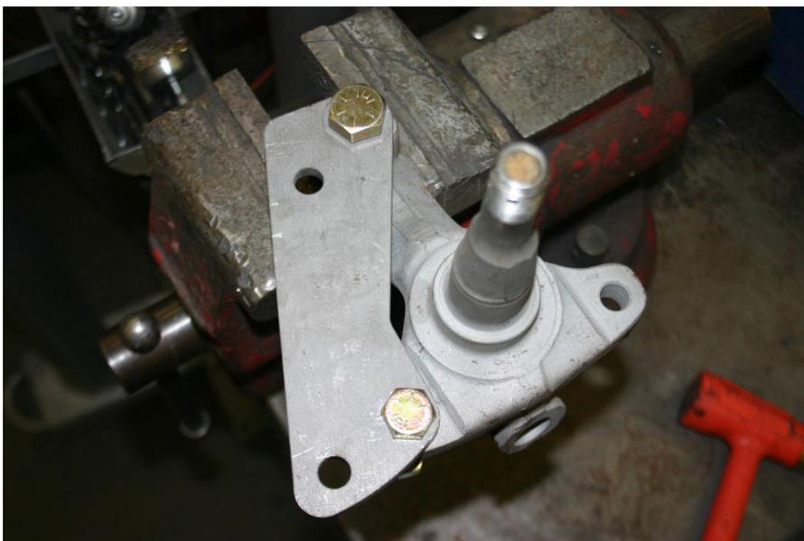
You will need to use the supplied ½" x 3" bolt in the rear steering arm bolt hole as the extra thickness of the bracket will make the factory one to short.
