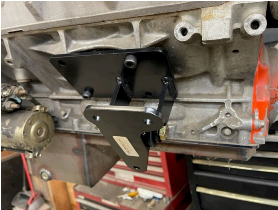
View of Passenger side engine and frame mount (note orientation of engine and frame mount)
